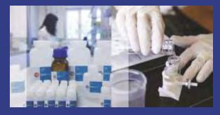
Legipid<sup>®</sup> test kit comes with all you need to run Legionella tests, apart from the PrimeLab plastic adapter for 1ml vials and a filter kit to filter your water sample.
